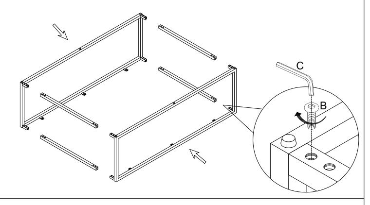
STEP 2:Use the Hex Key(C) to assemble the Connect Tube (C3) to the Top Panel (C1) with Bolt (A).
